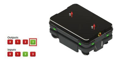
b. Once the pins are raised, verify that **3** under **Inputs** is green.
