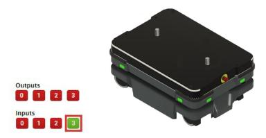
c. Under Outputs, select 2. Verify that the carrier pins lower into the robot.
