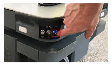
The status lights waver yellow, and the robot starts the software initialization process.
