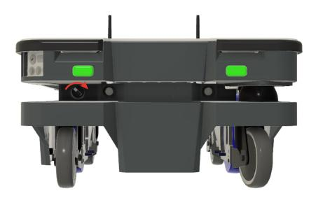
The mechanical brakes require electrical power to be released, so if the robot is without power, the mechanical brakes cannot be released.
