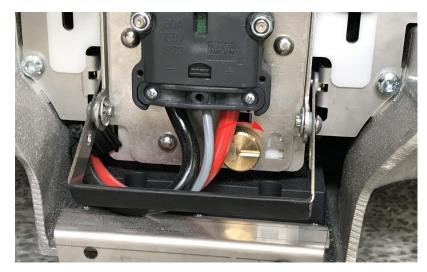
2. Pull up the lever to connect the battery connector to the battery. Then turn the battery lever lock counterclockwise to secure the battery lever.
