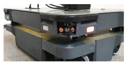
4. When the robot finishes the shutdown process, the status and the signal lights go off, and the Power button turns blue.
