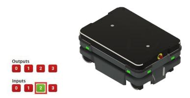
If the pins were raised and lowered as expected and the correct input feedback was received, the MiR Shelf Carrier 250 is correctly installed.
